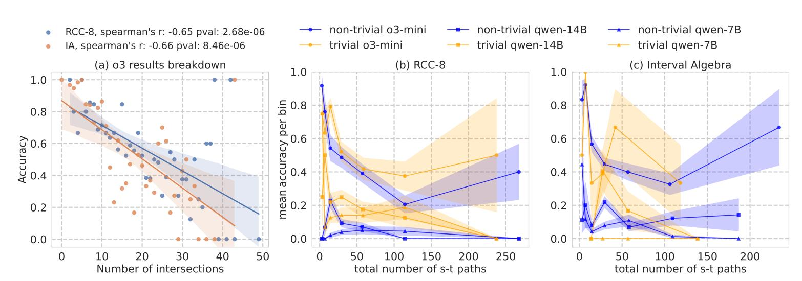
LRMs are shallow Algebraic Closure Algorithm (ACA) simulators. (a) o3-mini's performance on STaR. (b)-(c) Models, increasingly with size, zero-shot exploit the trivial path heuristic for solving STaR problems. Error bars are  $\pm 1\sigma$ .
