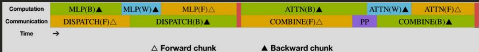
Figure 4: Overlapping strategy for a pair of individual forward and backward chunks (the boundaries of the transformer blocks are not aligned). Orange denotes forward, green denotes "backward for input", blue denotes "backward for weights", purple denotes PP communication, and red denotes barriers. Both all-to-all and PP communication can be fully hidden.
